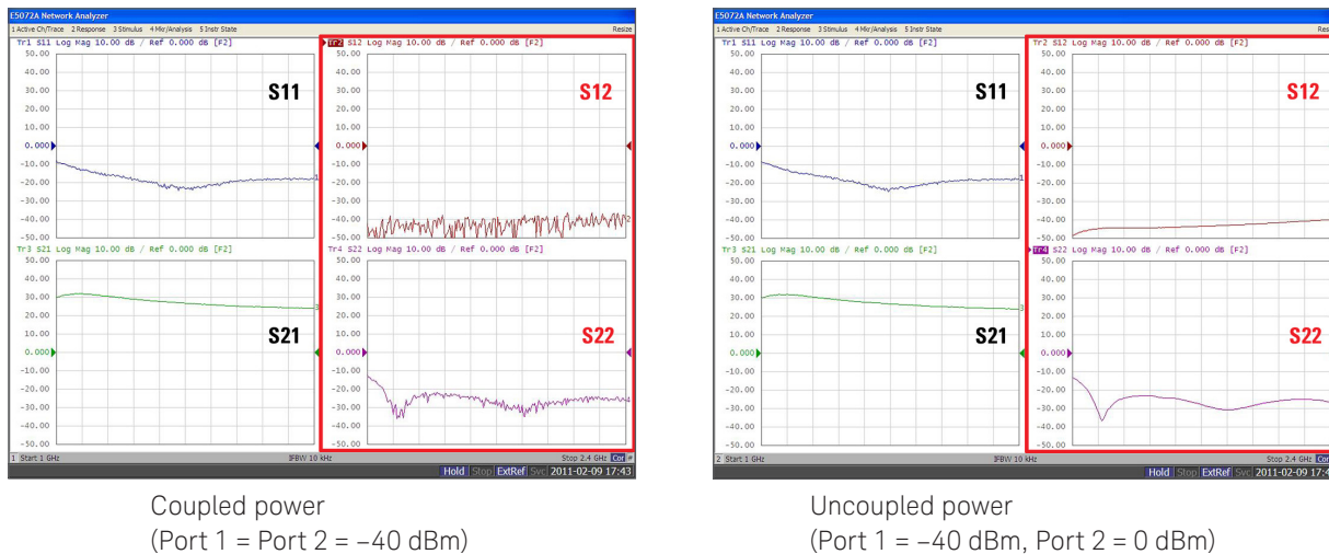
Figure 10. Uncoupled power improved the accuracy of measurement of high-gain amp
